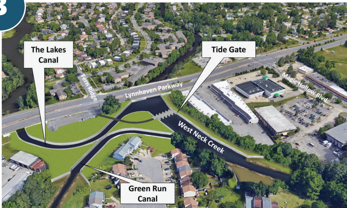
Rendering of Potential South London Bridge Creek Tide Gate & Channelization
